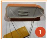
The two center wires are twisted together to turn the sensor on and then the protective tape seals the connection.
