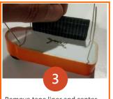
Remove tape liner and center the foam tape over the connection
